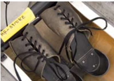
LEATHER FOOT BRACES WITH HEEL CUPS ADJUST TO DIFFERENT FOOT SIZES
